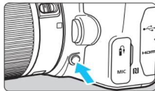
Press the depth-of-field preview button to stop down the lens to the current aperture setting and check the depth of field (range of acceptable focus).
