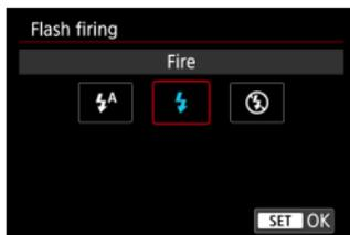
Set to [**⚡<sup>A</sup>**] to have the flash fire automatically, based on shooting conditions.
