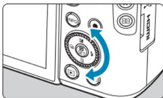
Turning the control dial is one way to choose setting items, switch images, and perform other operations. Additionally, you can perform most of the operations that are possible with the <▲> <▼> <◀> <▶> keys.
