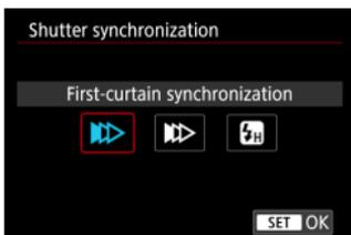
Normally, set this to **[First-curtain synchronization]** so that the flash fires immediately after the exposure starts.
