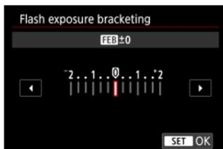
External Speedlites equipped with flash exposure bracketing (FEB) can change the external flash output automatically as three shots are taken at once.
