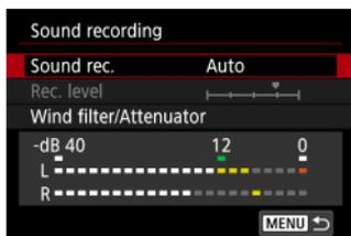
You can record movies while recording sound with the built-in stereo microphone or an external stereo microphone. You can also freely adjust the sound-recording level. Use [CAMERA]: **Sound recording** to set sound recording functions.
