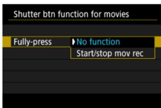
With [**Fully-press**] set to [**Start/stop mov rec**], you can start/stop movie recording not only by pressing the movie shooting button but also by pressing the shutter button completely or by using Remote Switch RS-60E3 (sold separately, 225).
