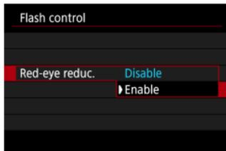
Set to [**Enable**] to reduce red-eye by emitting the red-eye reduction lamp before firing the flash.
