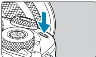
By pressing the <M-Fn> button and turning the <☀> dial, you can set the ISO speed.
