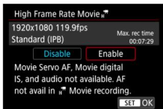
Movies are recorded as **[FHD 119.99 IPB]** or **[FHD 100.00 IPB]**. They are recorded cropped around the center of the shooting screen. Movie Servo AF and Movie digital IS have no effect when recording High Frame Rate movies. AF is not used to focus.
