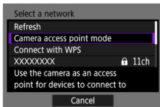
Camera access point mode is a connection mode for connecting the camera directly to each device via Wi-Fi.
