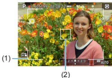
3. To move the AF point into position for focusing, press the button, then use the < dials or cross keys. Pressing the button will return the AF point to the screen center. You can also tap the screen to move the AF point.
