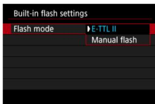
Set to [**E-TTL II**] to shoot in E-TTL II/E-TTL fully automatic flash mode.
