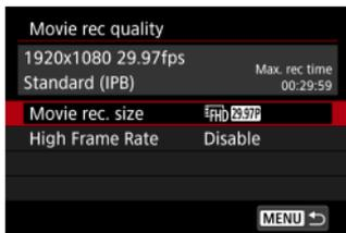
On the [**📷: Movie rec quality**] tab, select [**Movie rec. size**] to set the image size, frame rate, and compression method. The movie will be recorded as an MP4 file. The frame rate displayed on the [**Movie rec. size**] screen switches automatically depending on the [**📷: Video system**] setting (📖 504).
