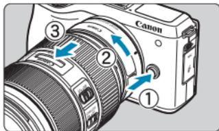
**1** While pressing the lens release button, turn the adapter as shown by the arrow.
