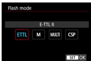
**[E-TTL II]** is the standard mode of EL/EX series Speedlites for automatic flash photography.
