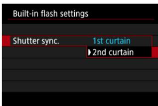
Normally, set this to **[1st curtain]** so that the flash fires immediately after the exposure starts.
