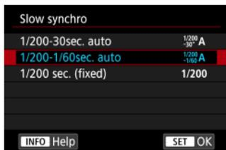
You can set the flash-sync speed for flash photography in <Av> aperture-priority AE mode or <P> Program AE mode.
