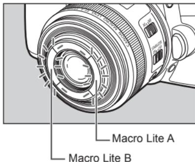
The Macro Lites on the front of the lens shine light on the subject during close-up (macro) photography to facilitate shooting. There are two light-emitting Macro Lites located on both sides of the lens, and it is possible to illuminate both simultaneously or either of them independently.
