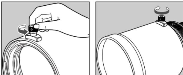
The dedicated Lens Hood ET-120 helps to prevent stray light from entering the lens and protects the front of the lens from rain, snow or dust.
