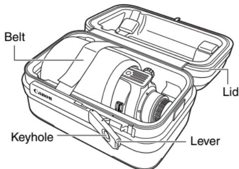
When putting the lens into its case, follow the procedure below.
