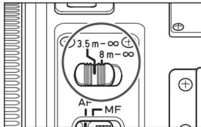
You can set the focusing distance range to 3.5 m/11.5 ft. to infinity or 8 m/26.2 ft. to infinity. By setting the suitable focusing distance range, the actual autofocus time can be shorter.
