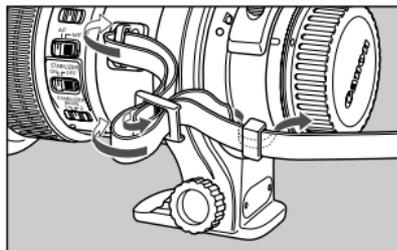
Thread the end of the strap through the strap mount on the lens and then back through the clasp on the strap. Pull the strap tight and check that there is no slack in the clasp.
