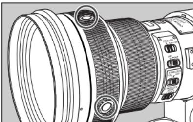
During autofocus operation, you can press the AF stop button to temporarily pause autofocus.
