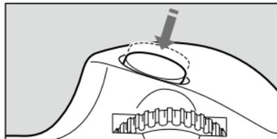
**1** After setting the zoom ring to macro, position the focusing ring so that the indicator appears in the center of the yellow line on the distance scale.
