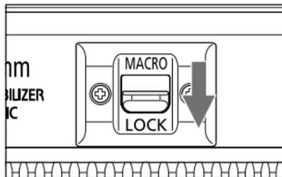
**2** Slide the zoom ring lock lever in the direction indicated by the arrow.
