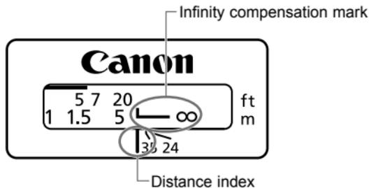
To compensate for shifting of the infinity focus point that results from changes in temperature. The infinity position at normal temperature is the point at which the vertical line of the distance scale L mark is aligned with the distance index.
