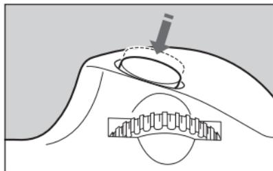
**3** Press the shutter button down halfway to enable stabilization (**MODE 1 and 2**).
