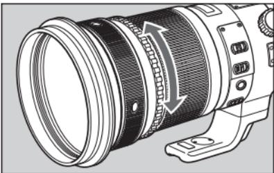
By turning the playback ring to the left or right, the focus shifts as far as the preset distance. Focus will shift freely released of AF focusing while the playback ring is still turned.
