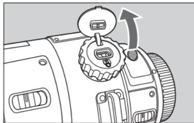
An attachment slot is provided for a wire-type security lock. The slot is located under the cover for the orientation locking knob.
