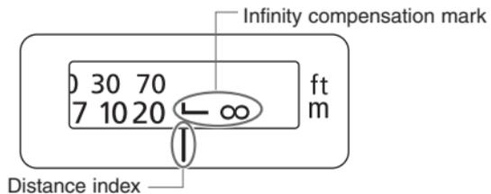
To compensate for shifting of the infinity focus point that results from changes in temperature. The infinity position at normal temperature is the point at which the vertical line of the L mark is aligned with the distance indicator on the distance scale.
