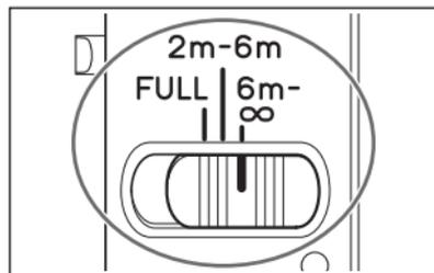
You can set the focusing distance range with a switch. By setting a suitable focusing distance range, the actual autofocus time will be shorter.
